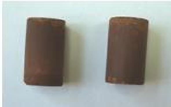
**Fig. 4 Sintered and cooled basalt parts**
